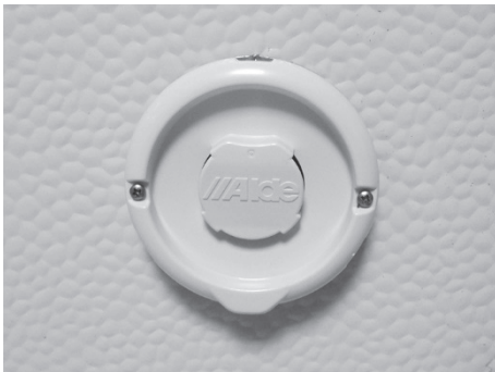
Fig. 85: Wall exhaust stack
