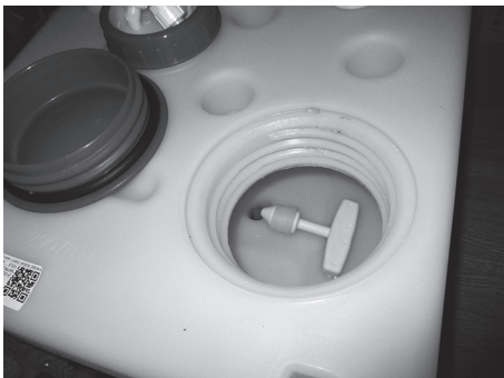
Fig. 95: Drain plug in the fresh water tank
