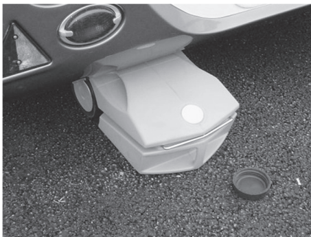
Fig. 109: Wheeled waste water tank
