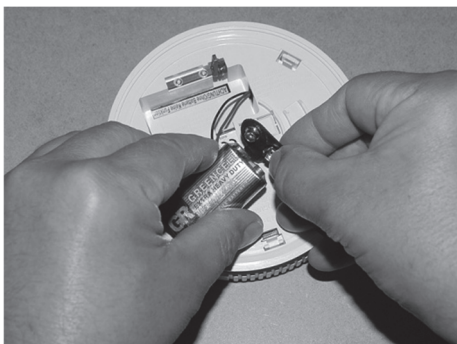
Fig. 206: Replacing the block battery
