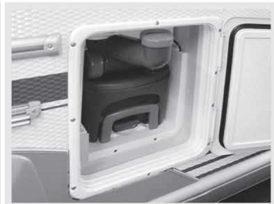
Fig. 50: Holding tank with flushing water intake port
