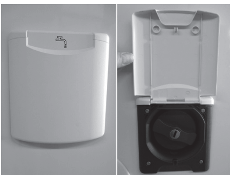
Fig. 23: Fresh water intake port
