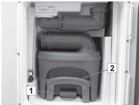
Fig. 172: Waste holding tank in the disposal shaft
